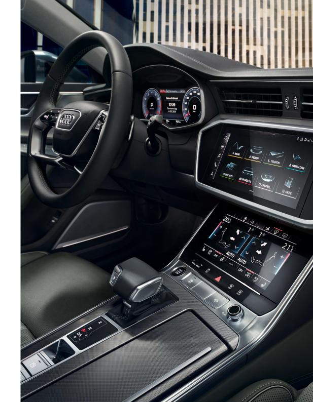
The MMI touch response operating concept offers the benefits of simple, intuitive control in the style of a smartphone and is safe to use even while driving thanks to touch feedback.
